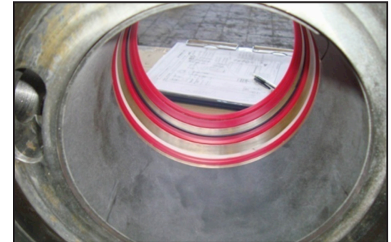
Chesterton rod seal system installed.
